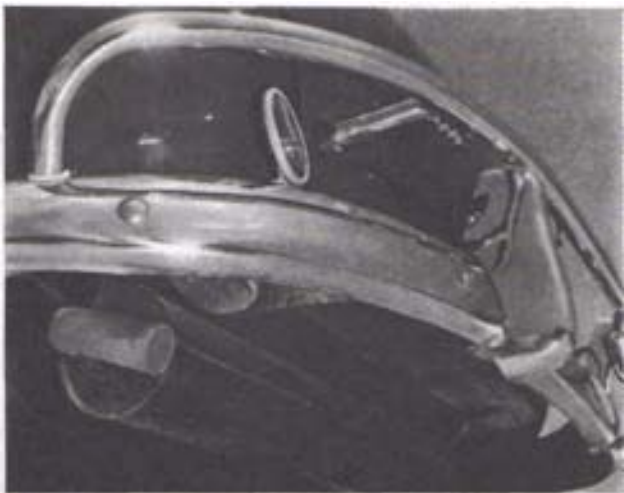
Bumper bracing is for U.S.-style bash and smash parking.
